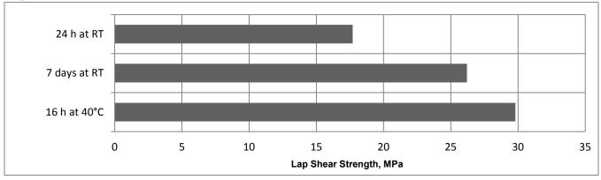
Average lap shear strengths of typical plastic-to-plastic joints (ISO 4587) (typical average values) Cured for 16 hours at 104°F (40°C) + 1 hour at 176°F (80°C) and tested at 73°F (23°C). Pretreatment - Lightly abraded and alcohol degreased.
